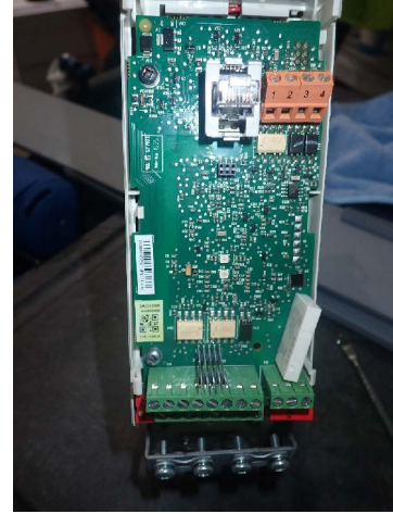
▲ ABB Variable frequency drive (VFD) drive after decontamination
