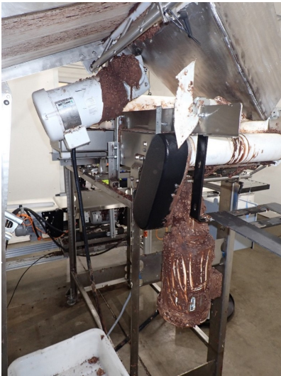
▲ AASTED metal detector and conveyor before decontamination
