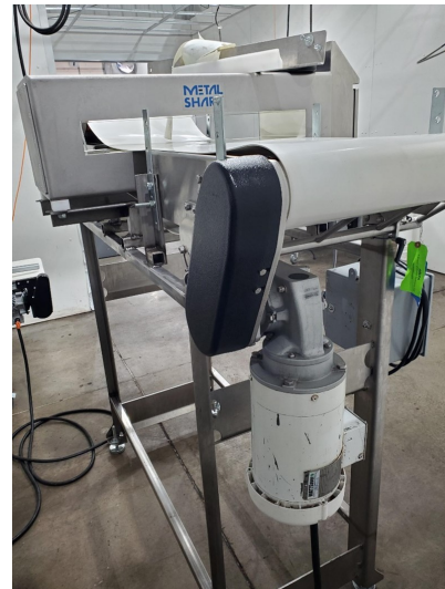
▲ AASTED metal detector and conveyor after decontamination
